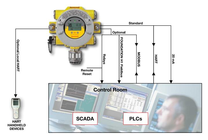
The XNX enclosure is available in a painted stainless steel or aluminum housing with a marine grade coating. Five threaded conduits/cable entries are available in Metric or NPT versions, and ruggedized mounting options provide ultimate installation flexibility. Instrumentation built on various sensing technologies can be attached locally to the transmitter or remotely with the appropriate
